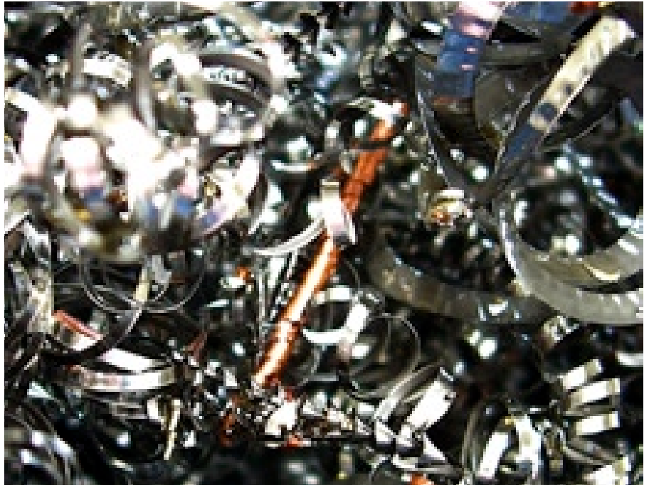
An excessive level of copper in steel scrap undermines the confidence in scrap as a raw material.
